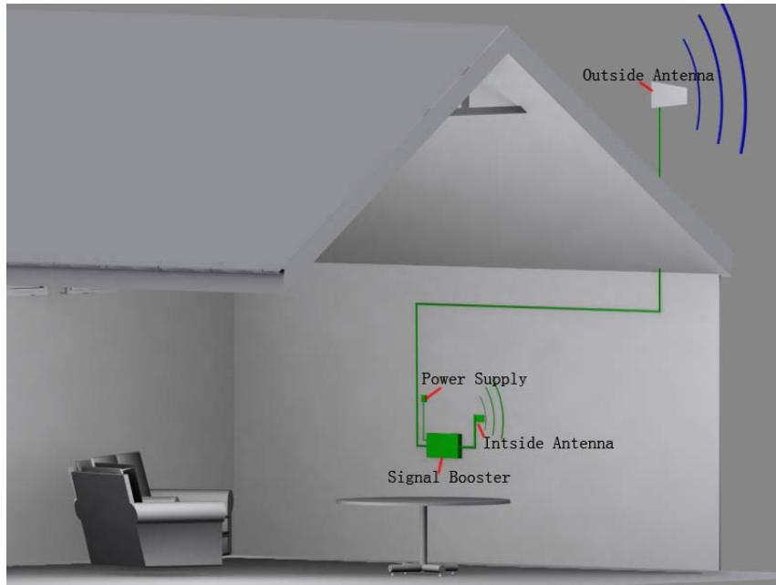
Indoor antenna gain $\leq$ 5dBi, without RF cable
