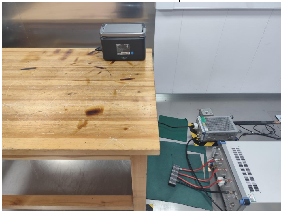
Conducted Emission at AC power line
