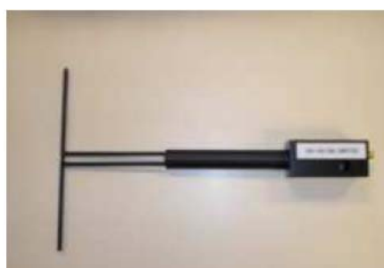
Figure 1 – Satimo COMOSAR Validation Dipole
