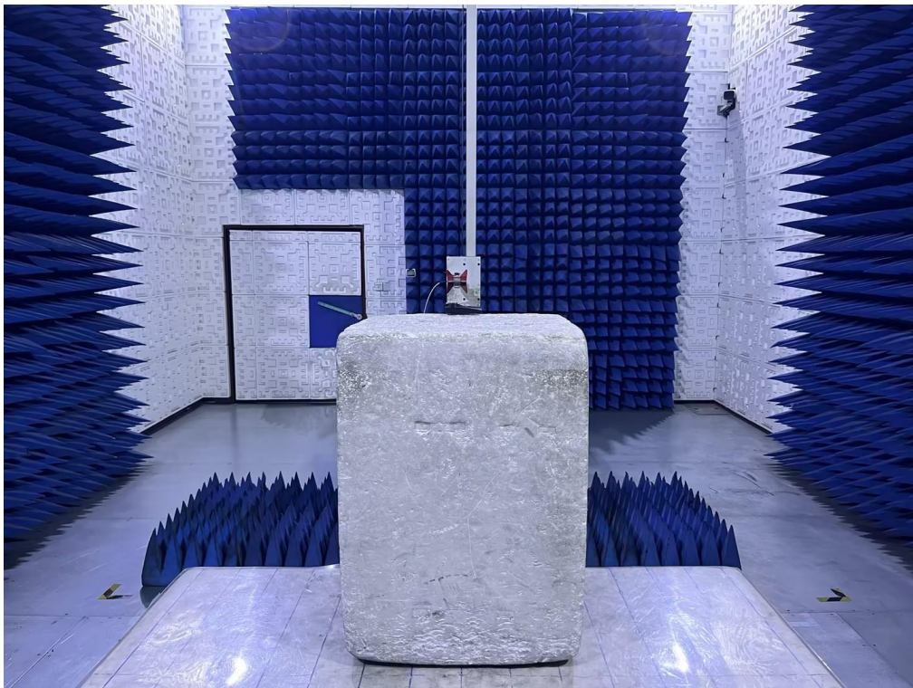
RADIATED EMISSION TEST SETUP ABOVE 1GHz
