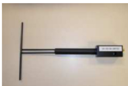
Figure 1 – Satimo COMOSAR Validation Dipole
