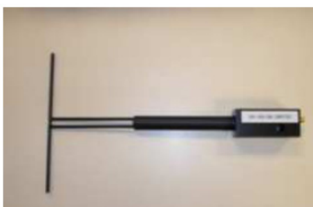
Figure 1 – Satimo COMOSAR Validation Dipole
