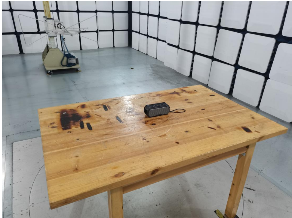
Photo of Radiation Emission Test
