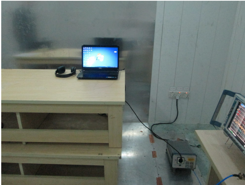
FCC RADIATED EMISSION TEST SETUP
