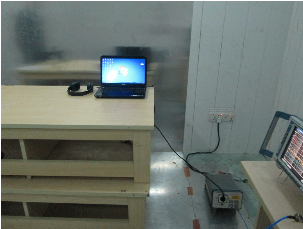
FCC RADIATED EMISSION TEST SETUP
