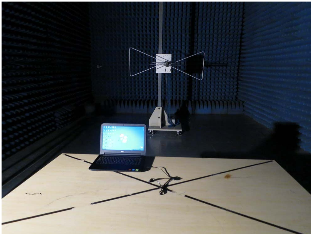
FCC RADIATED EMISSION TEST SETUP
