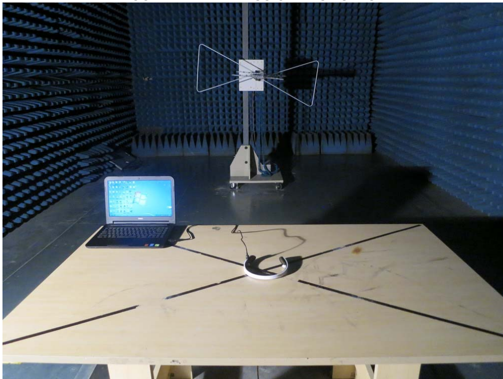
FCC RADIATED EMISSION TEST SETUP
