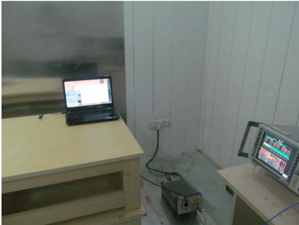
FCC RADIATED EMISSION TEST SETUP
