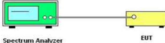
The EUT which is powered by the Battery, is connected to the Spectrum Analyzer; the RF load attached to the EUT antenna terminal is 50 Ohm; the path loss as the factor is calibrated to correct the reading. Make the measurement with the spectrum analyzer's resolution bandwidth(RBW) = 100 kHz. In order to make an accurate measurement, set the span greater than RBW.
