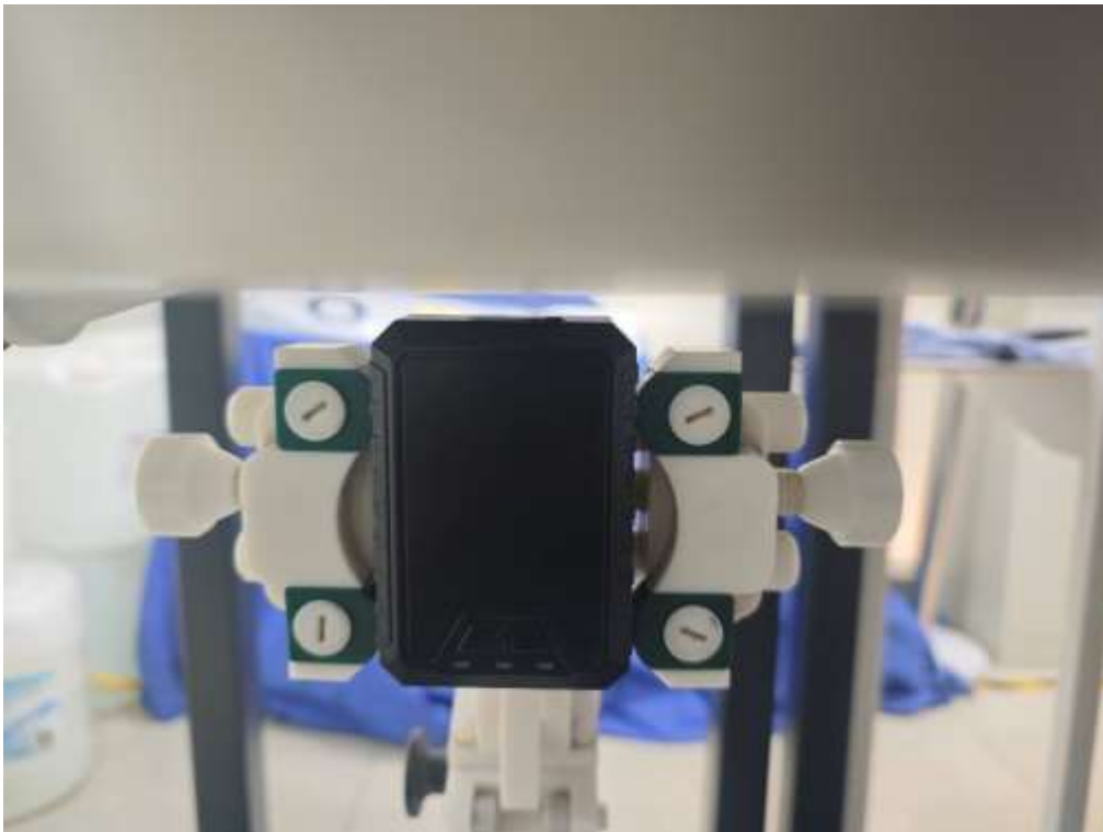
Body Bottom side(separation distance is 5mm)
