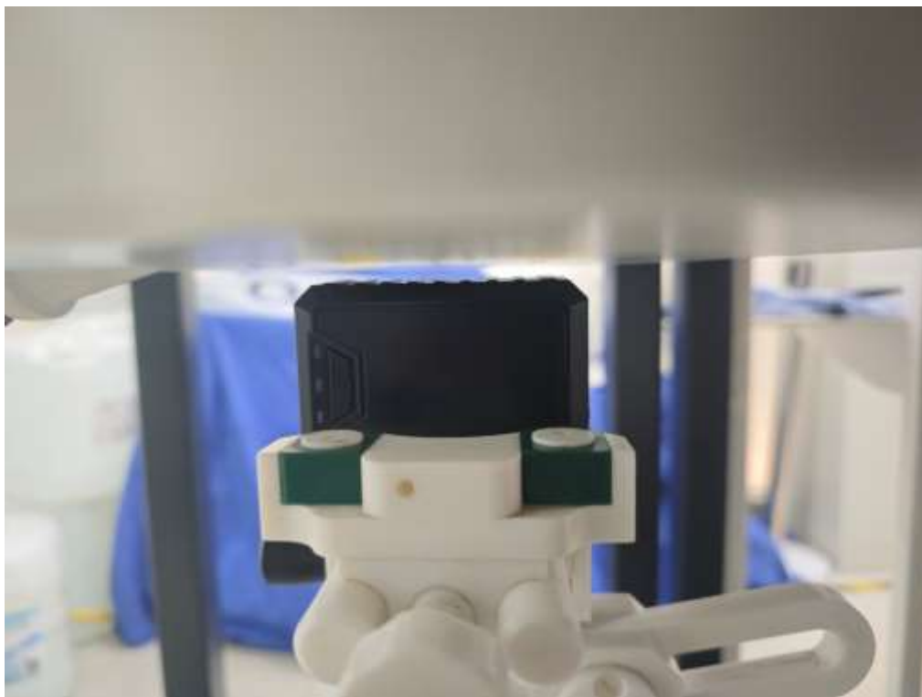
Body Right side(separation distance is 5mm)
