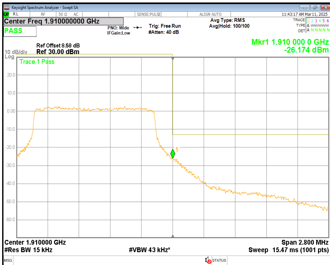
Band2 16QAM BW=3MHz Channel=18615 RB Size=15 Position=#0
