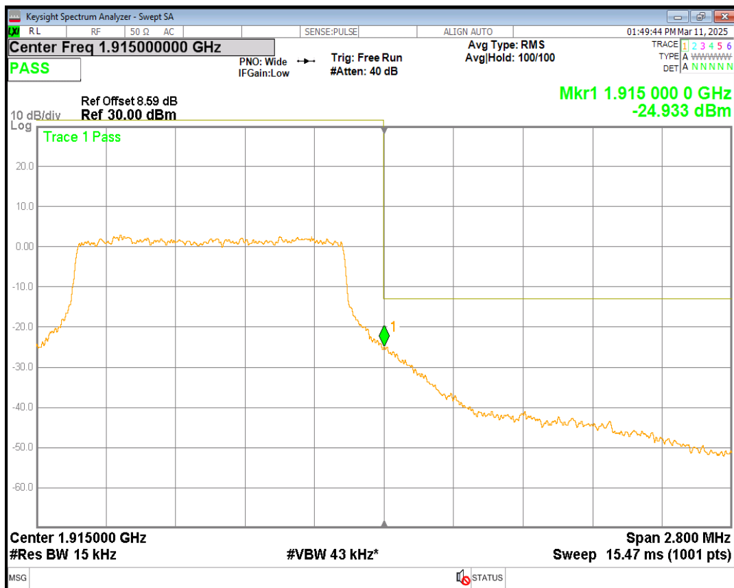
Band25 16QAM BW=3MHz Channel=26055 RB Size=15 Position=#0
