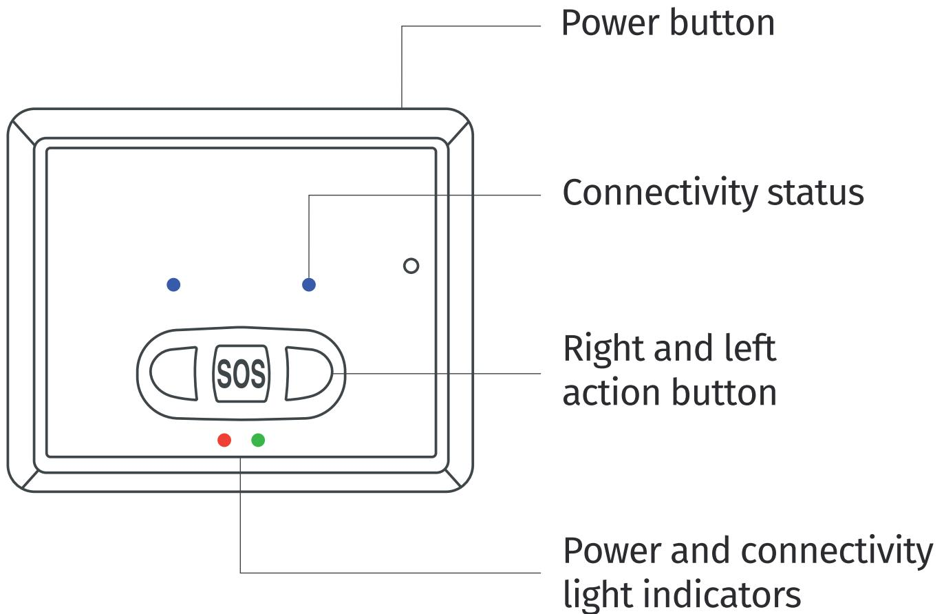
\* GPS Trackers need a clear view of the sky to properly receive signals and work best when the device is outdoors, and in or under the vehicle. Wi-Fi or cellular location will be used when the GPS signal is blocked by metal enclosures (i.e a trunk of a car), concrete, trees, heavy clouds and other interference factors.
