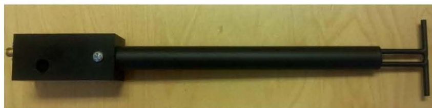
Figure 1 – MVG COMOSAR Validation Dipole
