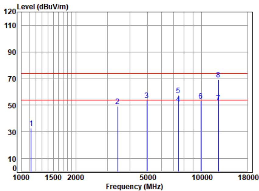
**Condition: 3m VERTICAL****Job No : 04038AT****Mode : 2480 TX RSE****: BLE 2M**
