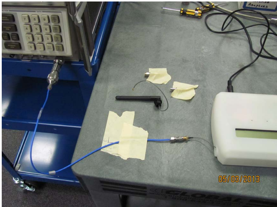
Photograph of Spurious Conducted Emissions Test Setup
