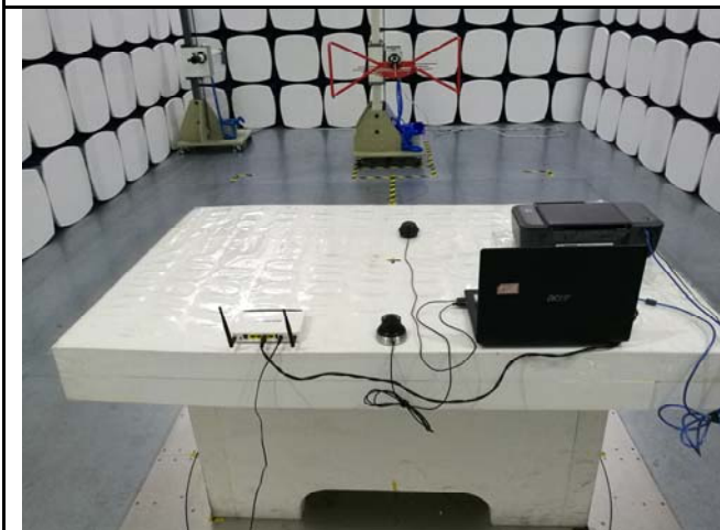
Radiated Emissions Test Setup Below 1GHz
