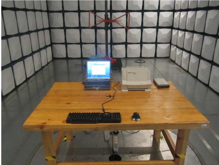
Radiated Emission - Front View (Below 1GHz)
