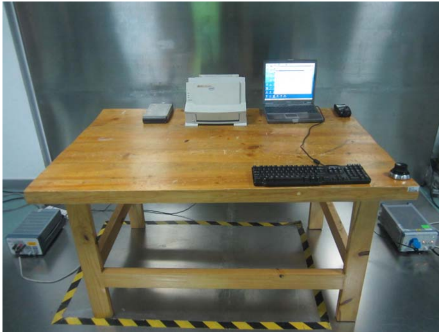
Conducted Emission - Front View
