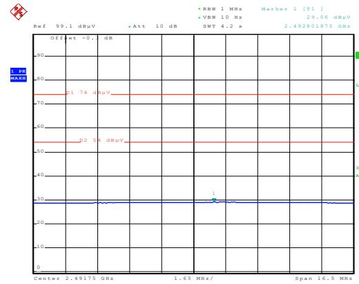
\* offset = Factor (ANT Factor+ Amp Gain + Cable Loss) [dB]
