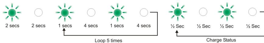
To switch off the Load Sensor while charging press the push switch for 1 second. The LED will do the following sequence to show it has turned off.
