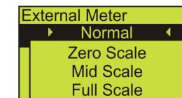
Used to calibrate any external meter connected to the analog output of the display. Use the UP and DOWN buttons to choose which function you want to test and press the OK button.
