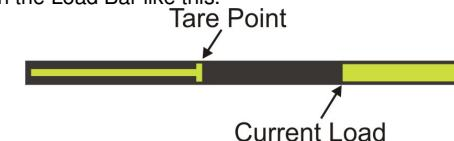
To set the tare again simply press the OK button with Tare Mode icon selected. To remove the tare either press and hold the OK button with Tare Mode icon selected or select normal mode icon and press OK.
