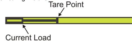
When load is applied and it takes the value above the tare point the display will show only the value of the additional load, **not** the combined load of the tare and additional load. This will be displayed on the Load Bar like this.
