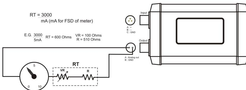
We advise putting a variable resistor in line with the fixed resistor to enable span calibration. To check the setup of your meter go to the meter output menu and select full, half and zero outputs and check that they read correctly on the meter, adjustments can be made via this variable resistor.
