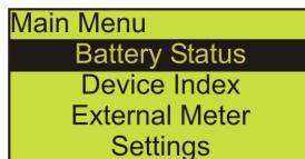
From this menu use the UP and DOWN buttons to scroll through the options: Battery Status, Device Index, External Meter, Settings and Exit. To select a sub menu click on the OK button.
