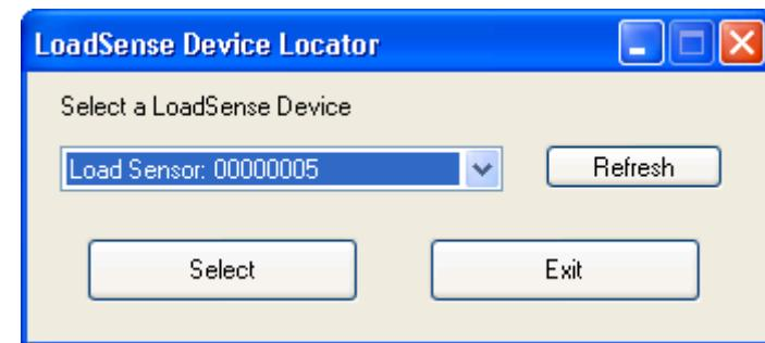
From the combo box select the load sensor that you want to use with the software and click "Select". If the load sensor is not listed check the connections and click "Refresh".
