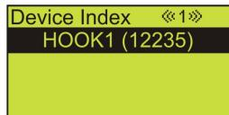
This section allows you to select which load sensor you want the display to show. If there are multiple sensors, use the up and down arrows to scroll through them and select one with the OK button.
