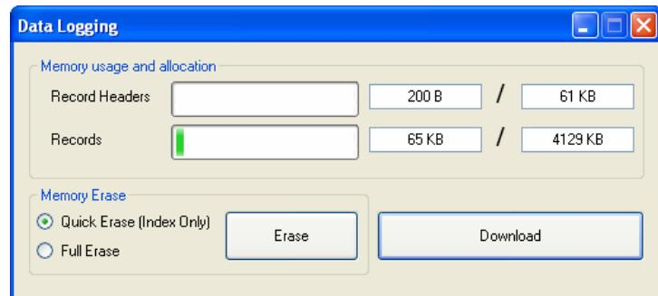
The internal memory is split into 3 sections, index, headers and records.
