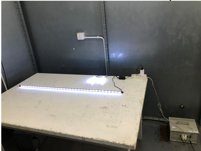
Measurement of Conducted Emission Test Set Up
