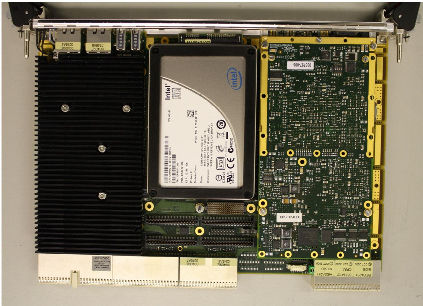
3d-Radar Geoscope cPCI computer Bottom View
