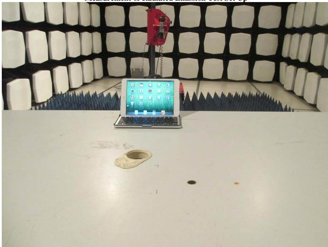
Measurement of Radiated Emission Test Set Up
