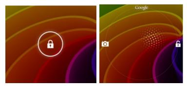
**Power saving & screen-lock:** turn on the device and short press"POWER" button to enter SLEEP power for saving mode, at this time, the screen become black screen, and also enter screen lock mode. Press "POWER" button again, the system resume bright screen within 1s.
