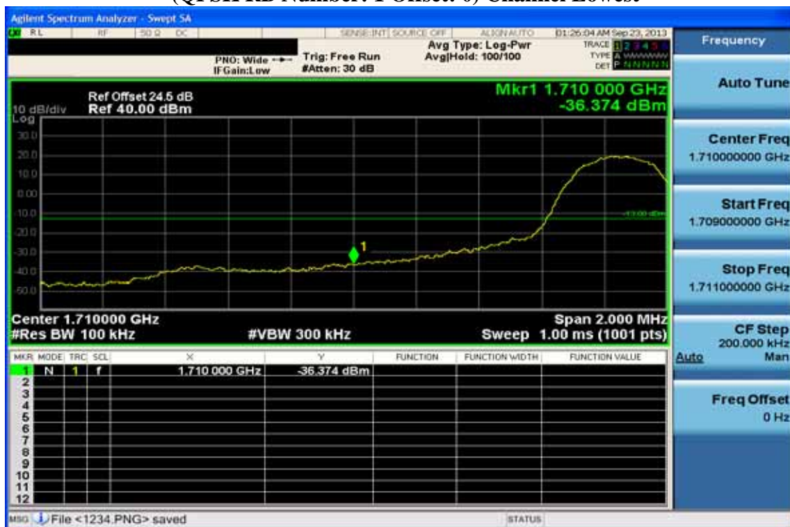
Figure 10-15: Band edge emission at antenna terminals –15MHz BW LTE-Band 4 (QPSK RB Number: 1 Offset: 74) Channel Highest
