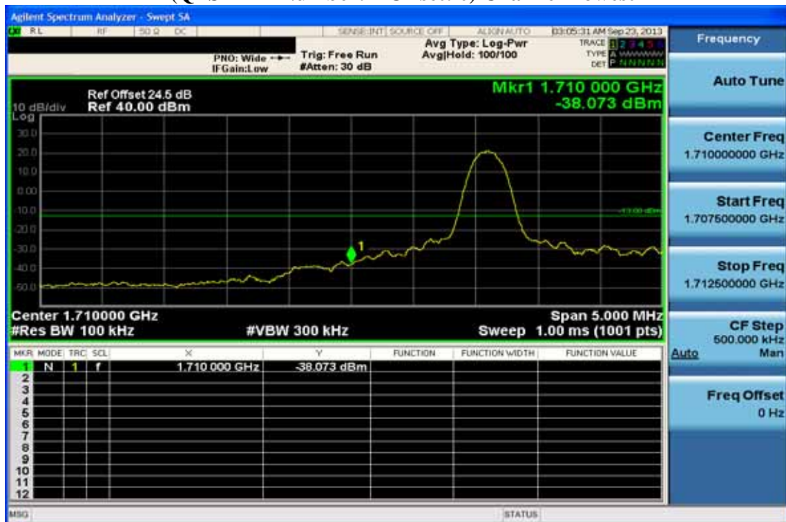
Figure 10-20: Band edge emission at antenna terminals –10MHz BW LTE-Band 4 (QPSK RB Number: 1 Offset: 99) Channel Highest
