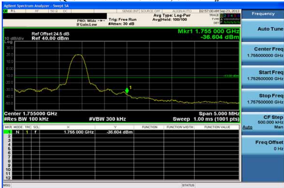
Figure 10-20: Band edge emission at antenna terminals –10MHz BW LTE-Band 4 (QPSK RB Number: 1 Offset: 99) Channel Highest
