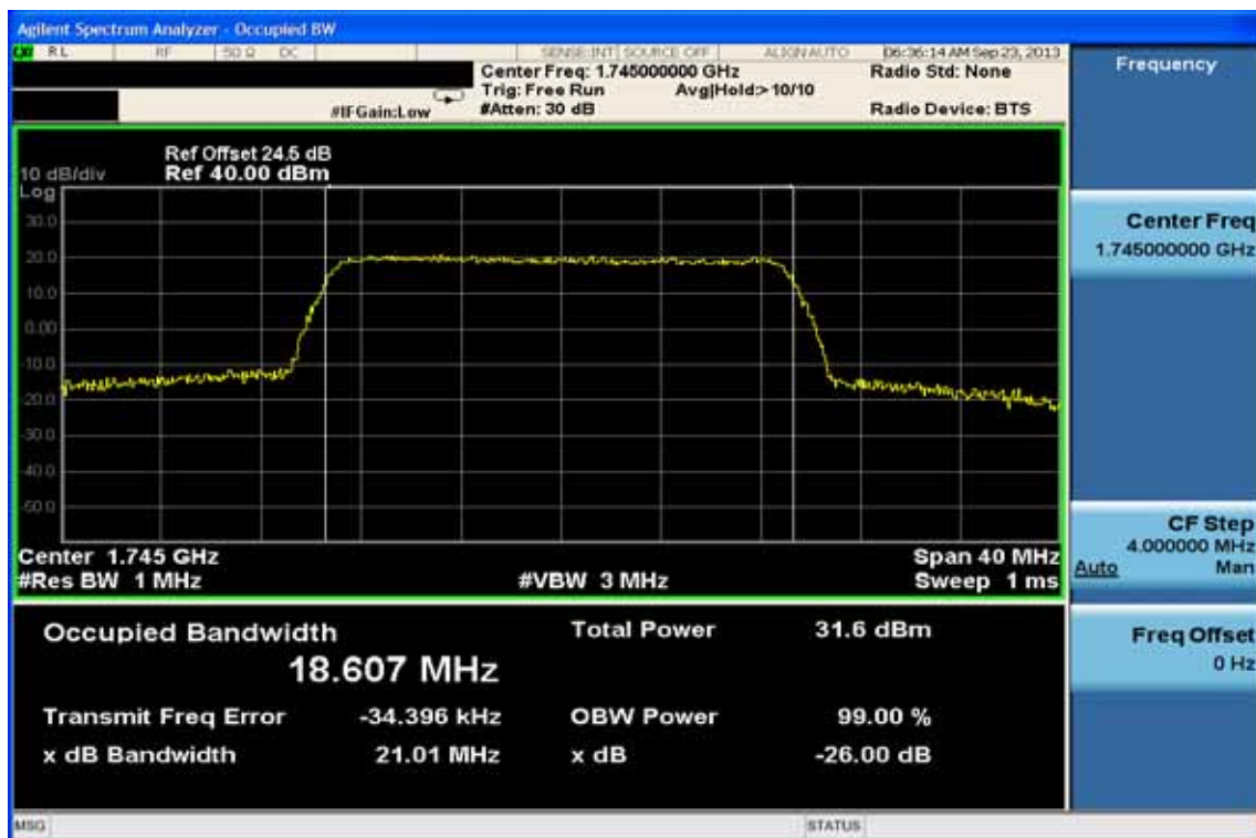
Figure 9-25: 20MHz BW LTE-Band 4(16QAM RB Number: 100 Offset: 0) Channel High
