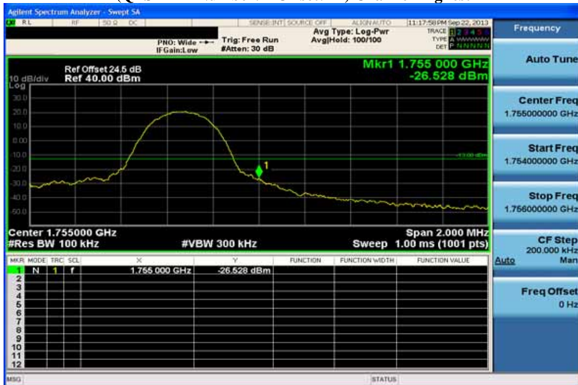
Figure 10-5: Band edge emission at antenna terminals –5MHz BW LTE-Band 4 (QPSK RB Number: 1 Offset: 24) Channel Highest
