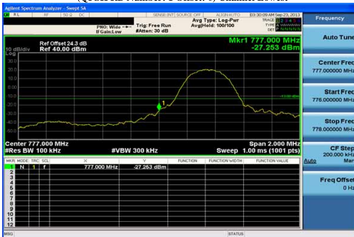
Figure 10-25: Band edge emission at antenna terminals –5MHz BW LTE-Band 13 (QPSK RB Number: 1 Offset: 24) Channel Highest
