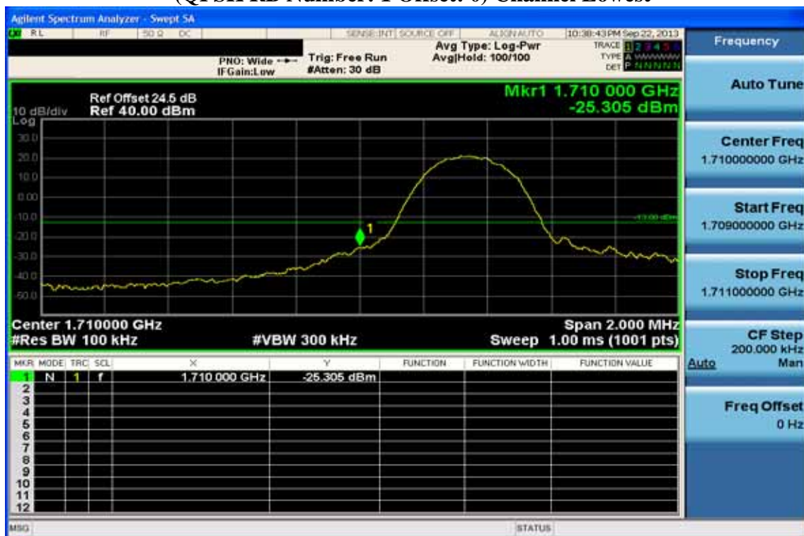
Figure 10-5: Band edge emission at antenna terminals –5MHz BW LTE-Band 4 (QPSK RB Number: 1 Offset: 24) Channel Highest
