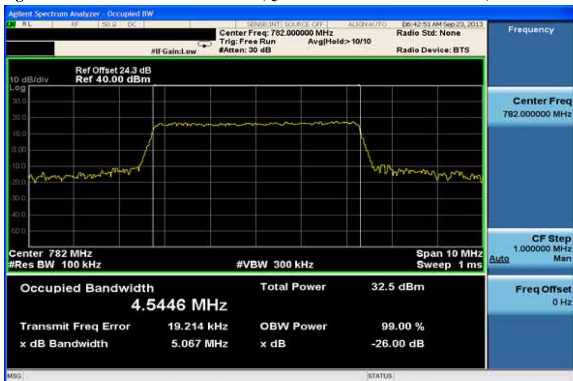
Figure 9-27: 5MHz BW LTE-Band 13(QPSK RB Number: 25 Offset: 0) Channel Mid
