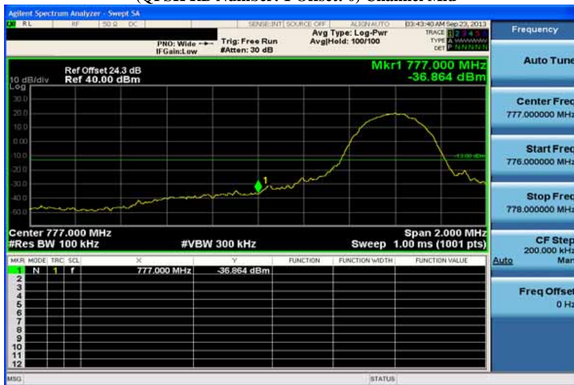
Figure 10-27: Band edge emission at antenna terminals –10MHz BW LTE-Band 13 (QPSK RB Number: 1 Offset: 0) Channel Mid
