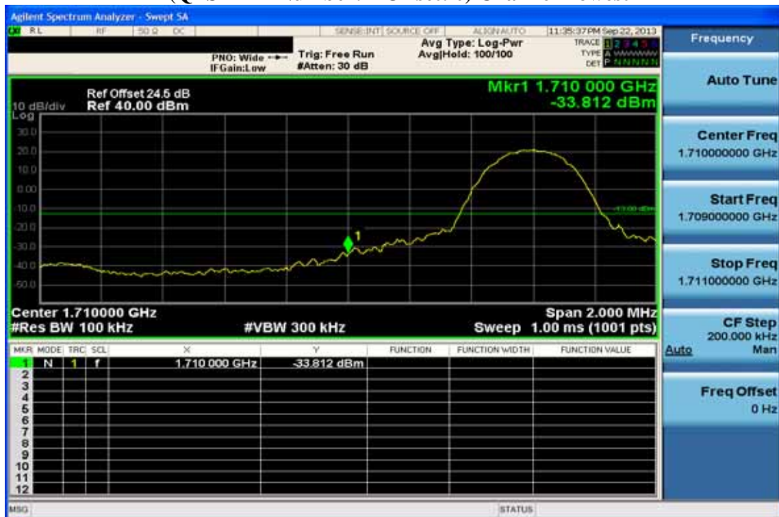
Figure 10-10: Band edge emission at antenna terminals –10MHz BW LTE-Band 4 (QPSK RB Number: 1 Offset: 49) Channel Highest
