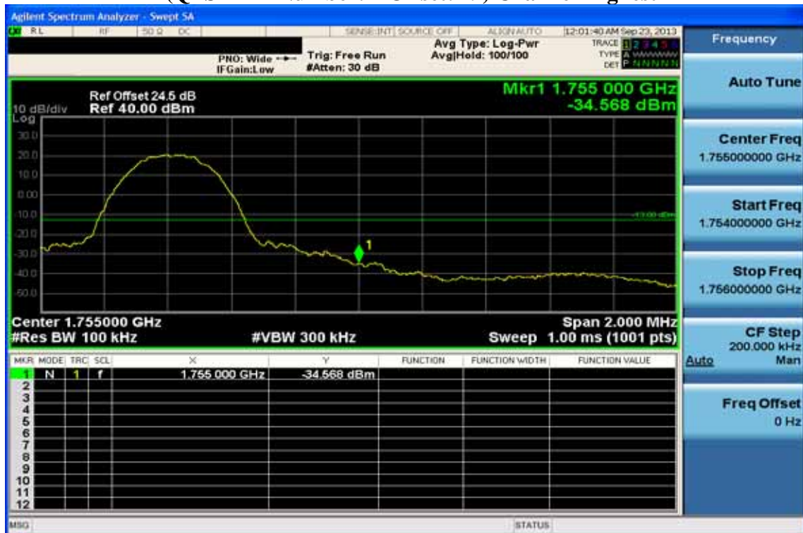
Figure 10-10: Band edge emission at antenna terminals –10MHz BW LTE-Band 4 (QPSK RB Number: 1 Offset: 49) Channel Highest
