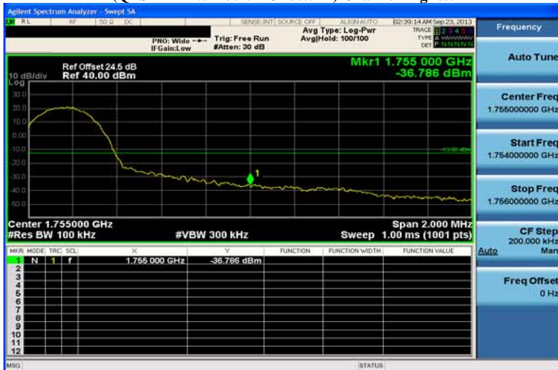
Figure 10-15: Band edge emission at antenna terminals –15MHz BW LTE-Band 4 (QPSK RB Number: 1 Offset: 74) Channel Highest
