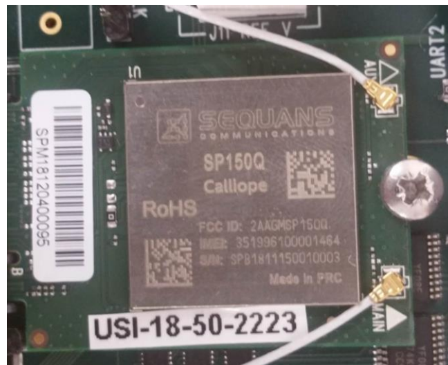
Figure B4. DUT Module (SP150Q) close view
