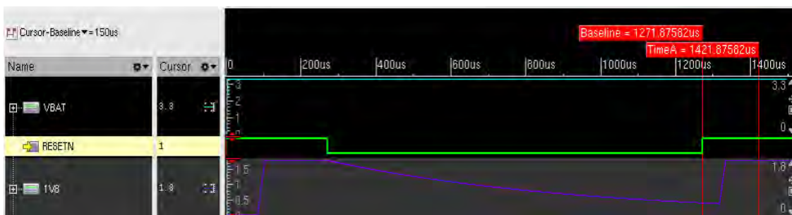
Figure 6. Typical Timing Diagram for Reset Sequence
