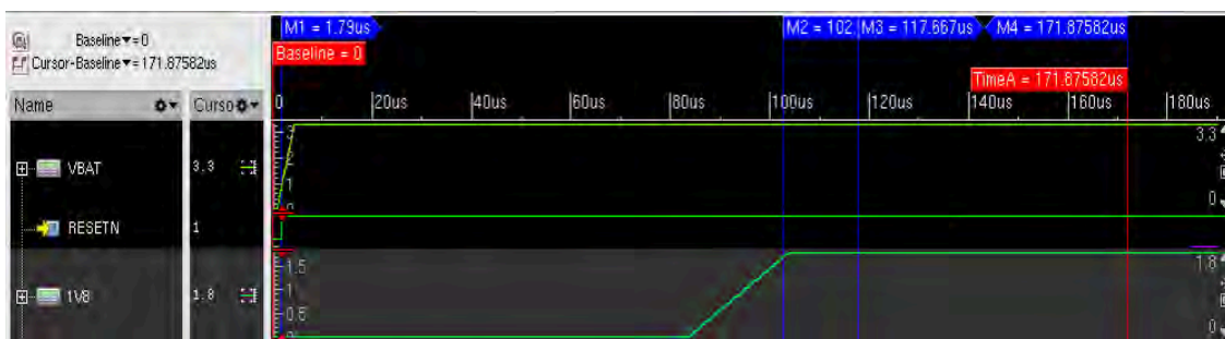
Figure 5. Typical Timing Diagram for Power-Up Sequence
