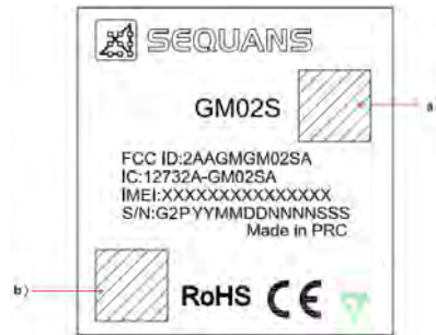
Figure 13. GM02S Laser Marking
