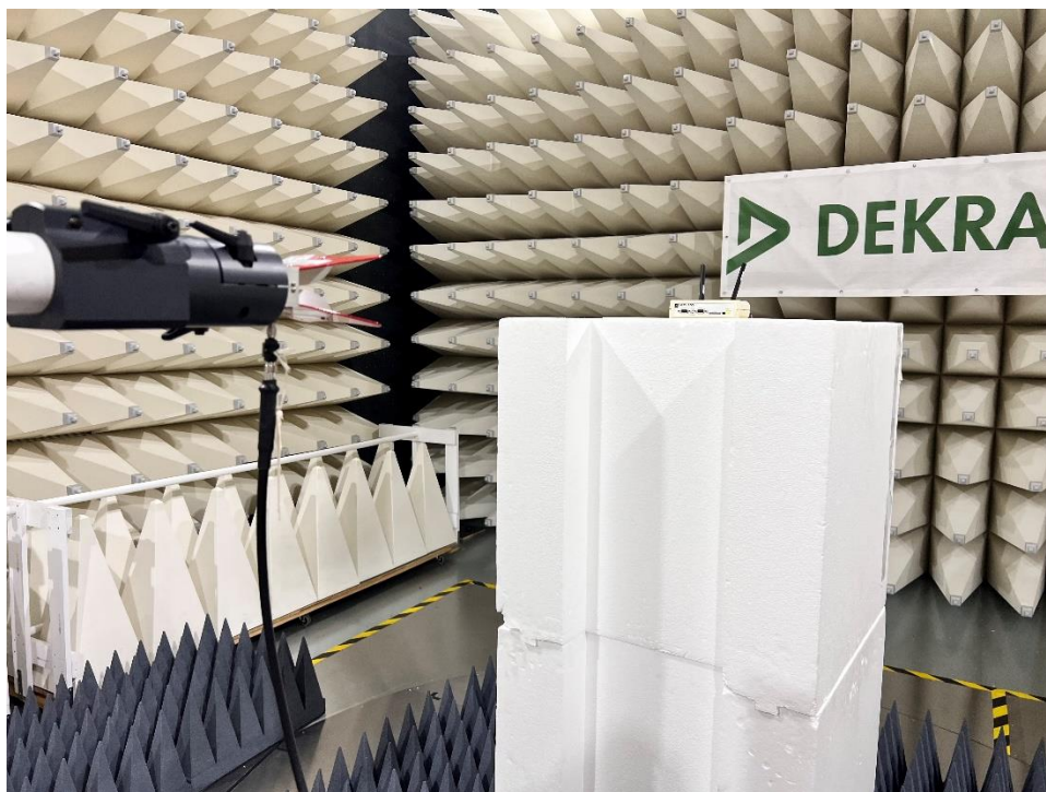
6. Radiated Emission test setup High Range 2
