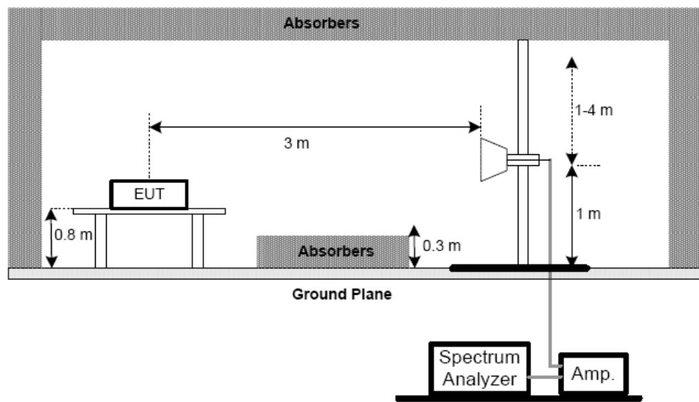
(C) For radiated emissions below 30MHz
