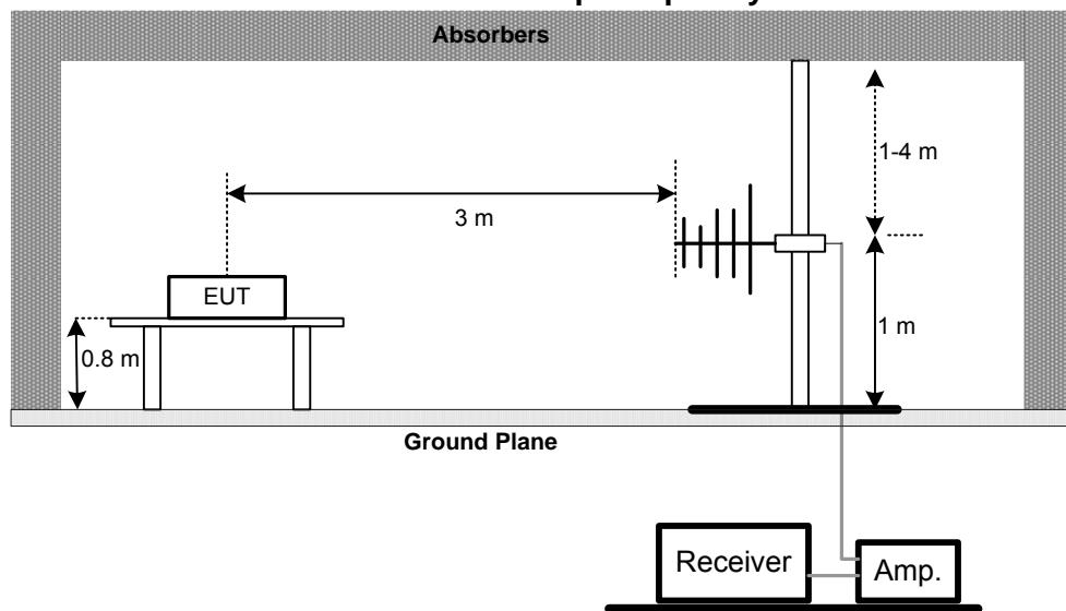
**Radiated Emission Test Set-Up Frequency Above 1 GHz**
