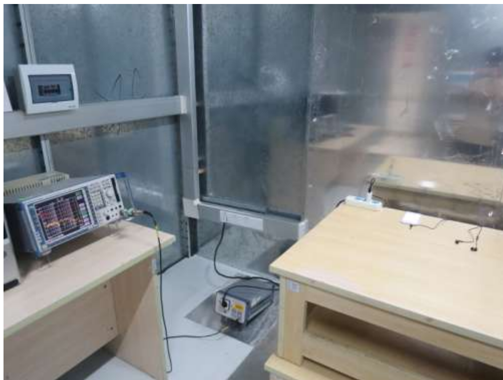
FCC RADIATED EMISSION TEST SETUP
