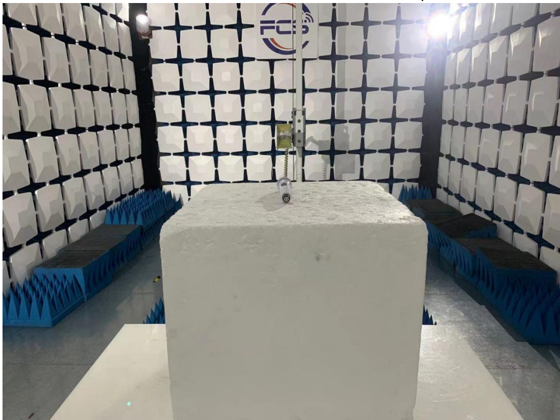
Above 1GHz for radiated emission test setup
