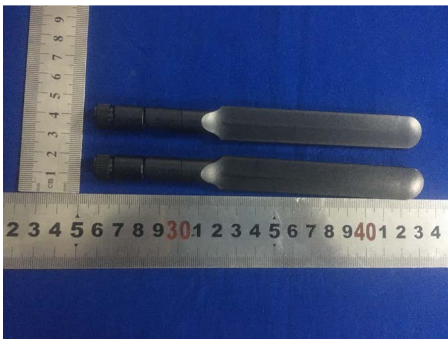
4G Antenna View
