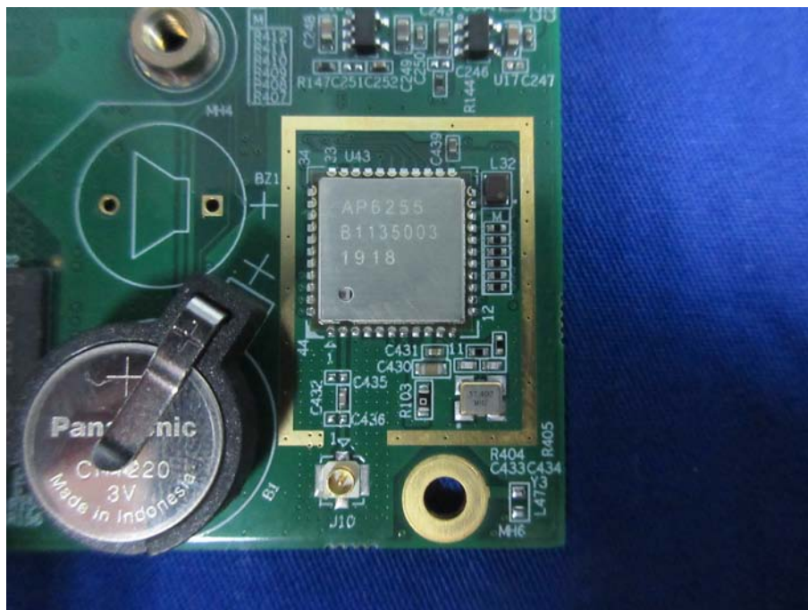
EUT –Wi-Fi & Bluetooth Module View
