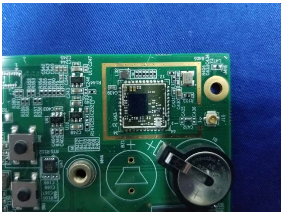
EUT –Wi-Fi & Bluetooth Module Shielding off View
