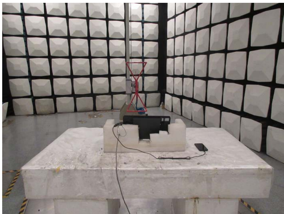
Radiated Emission View (Below 1GHz)-Powered by POE
