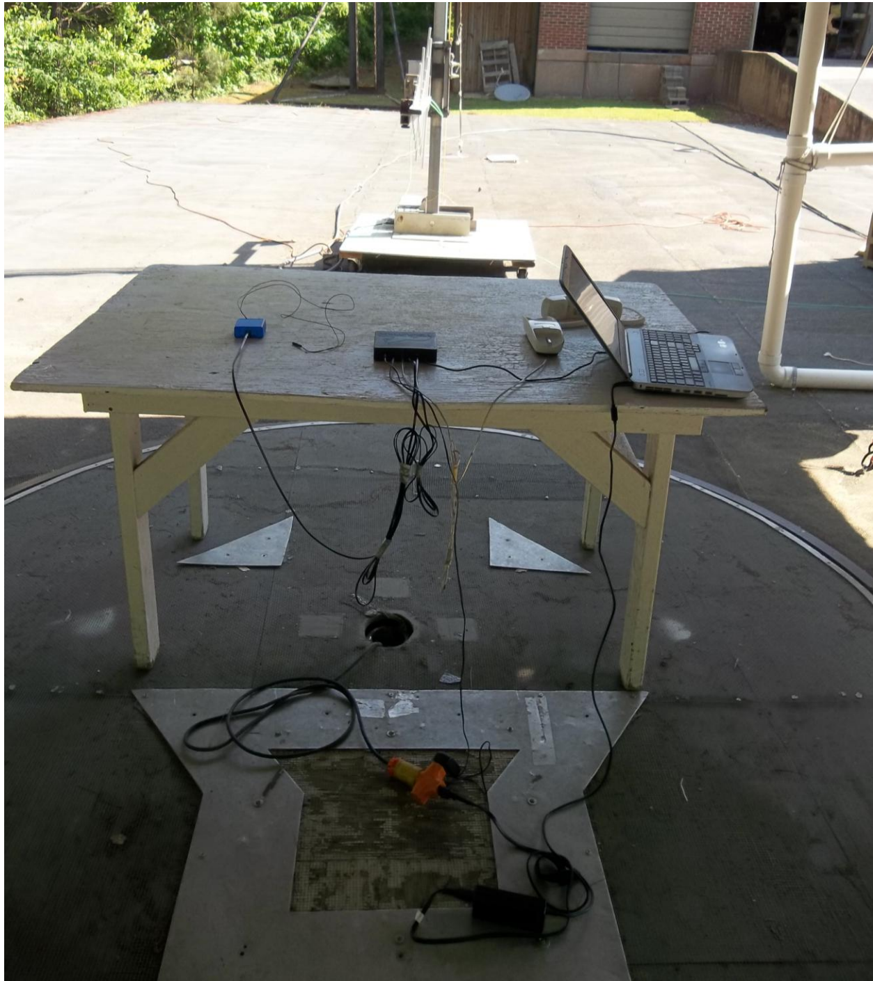
Rear View Radiated Emissions Test Setup with Log-Periodic Antenna
