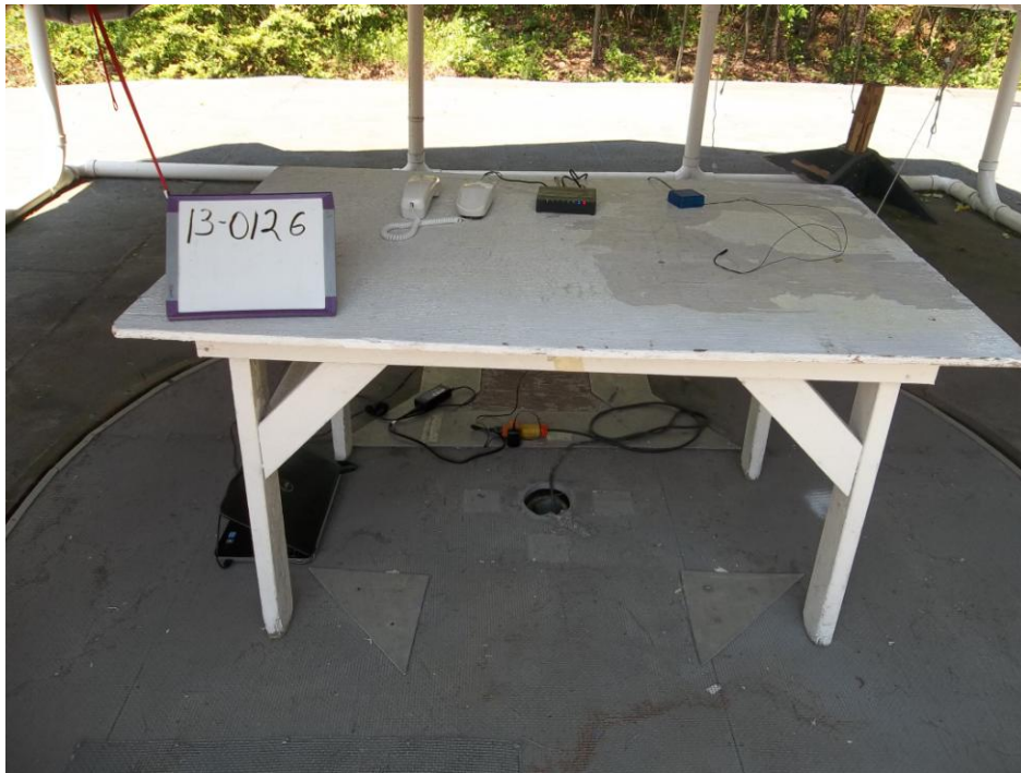
Front View Radiated Emissions Test Setup
