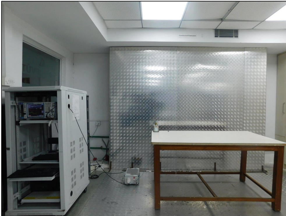
Test Setup of Conducted Emission on AC Power lines
