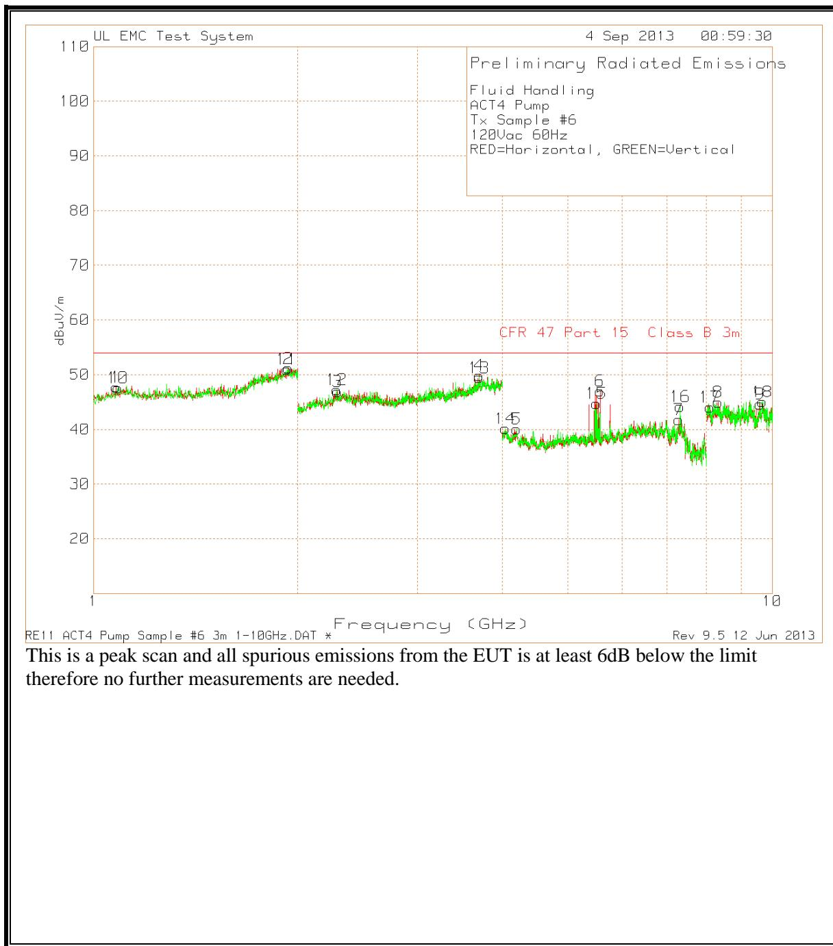
This is a peak scan and all spurious emissions from the EUT is at least 6dB below the limit therefore no further measurements are needed.
