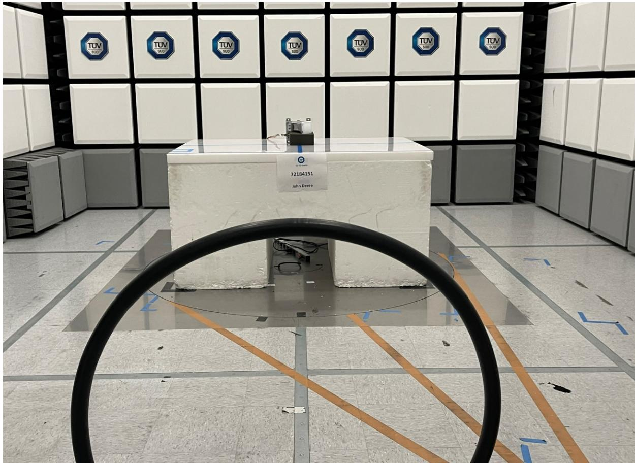
**Radiated Emissions Test Setup (below 30MHz)**
