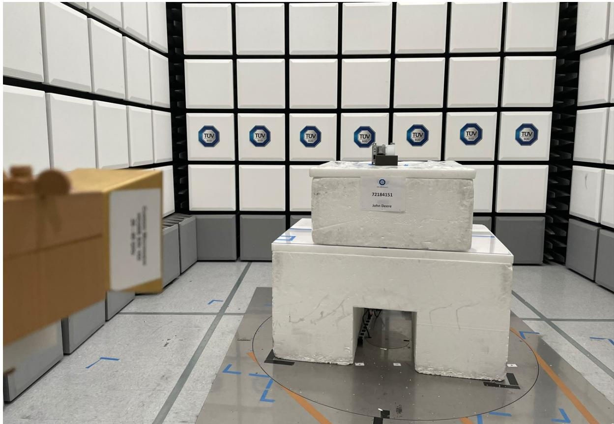
**Radiated Emissions Test Setup (26GHz to 40GHz)**
