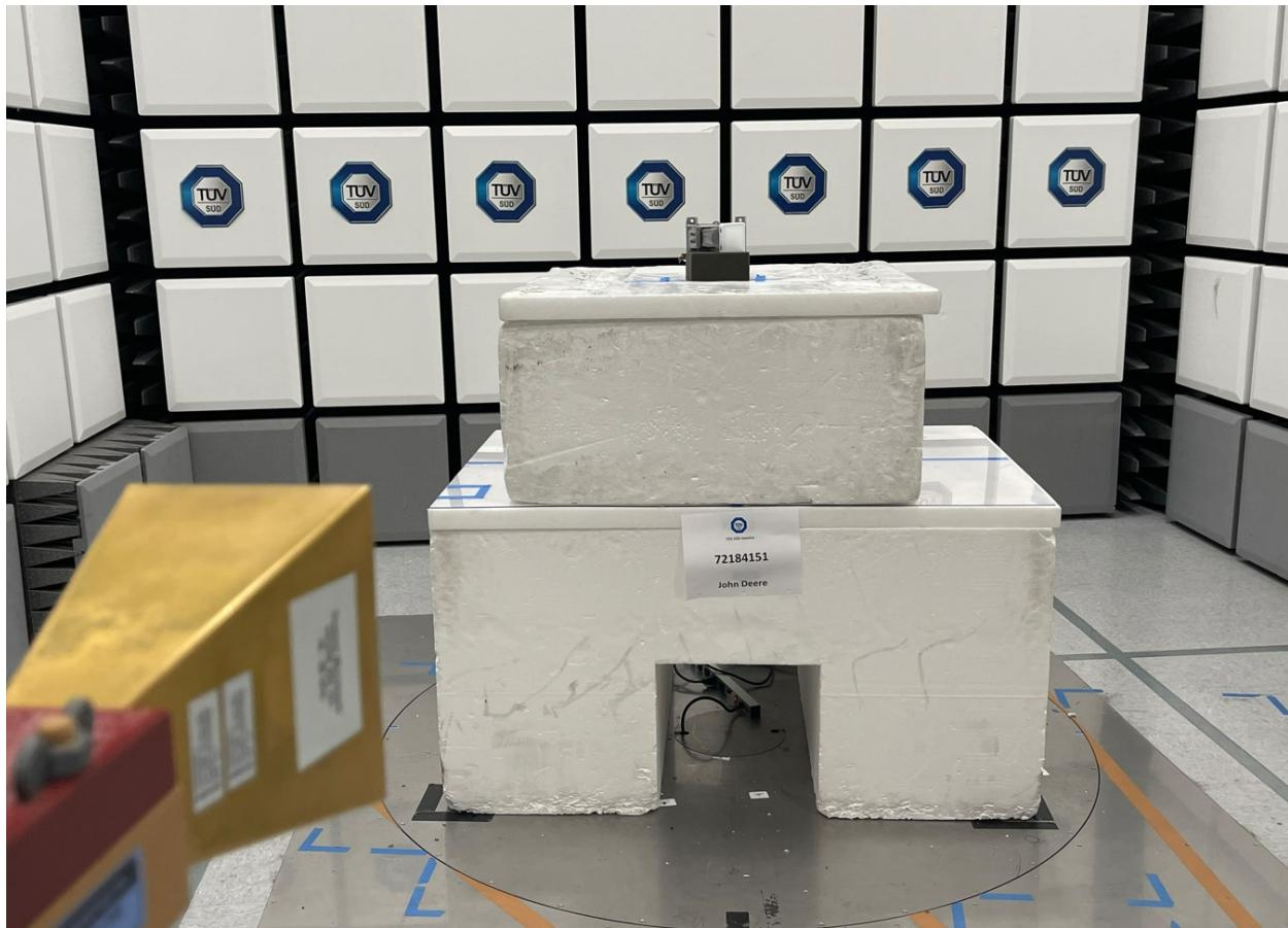
**Radiated Emissions Test Setup (18GHz to 26GHz)**
