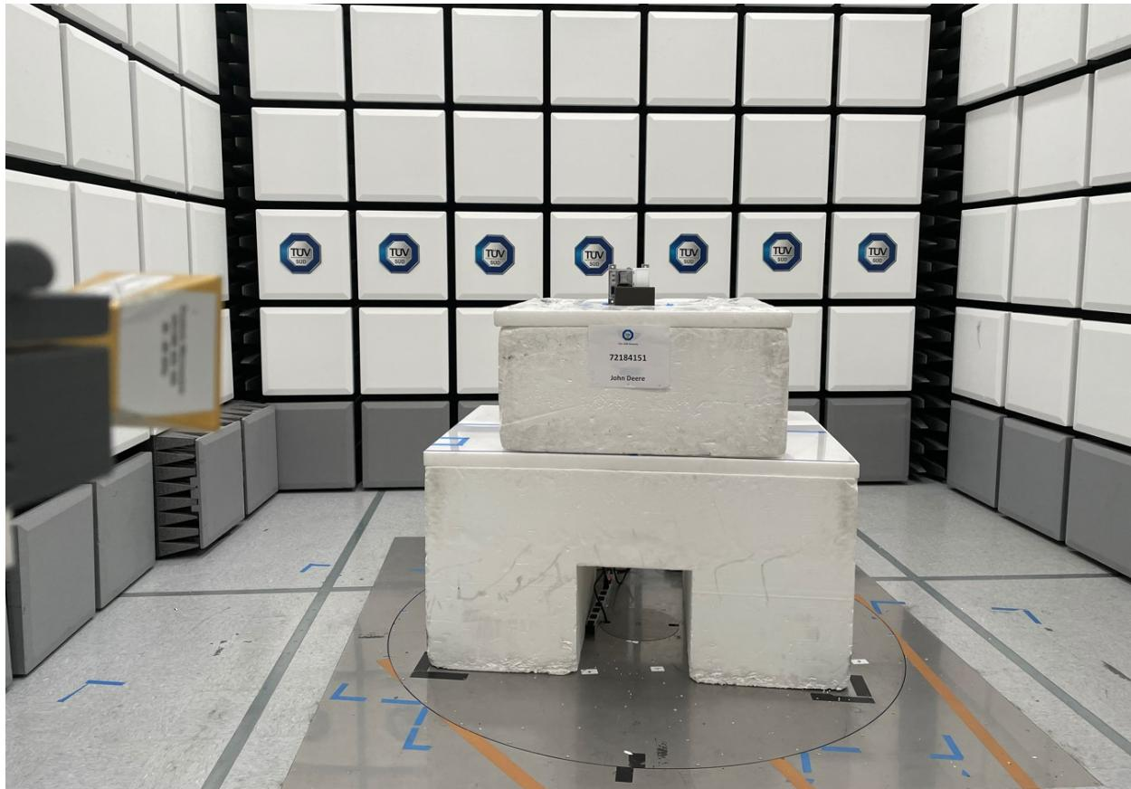
**Radiated Emissions Test Setup (above 40GHz)**
