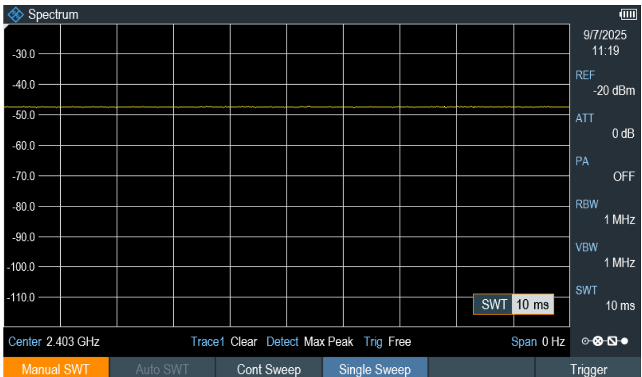
Time-domain plot for Bluetooth transmission signal
