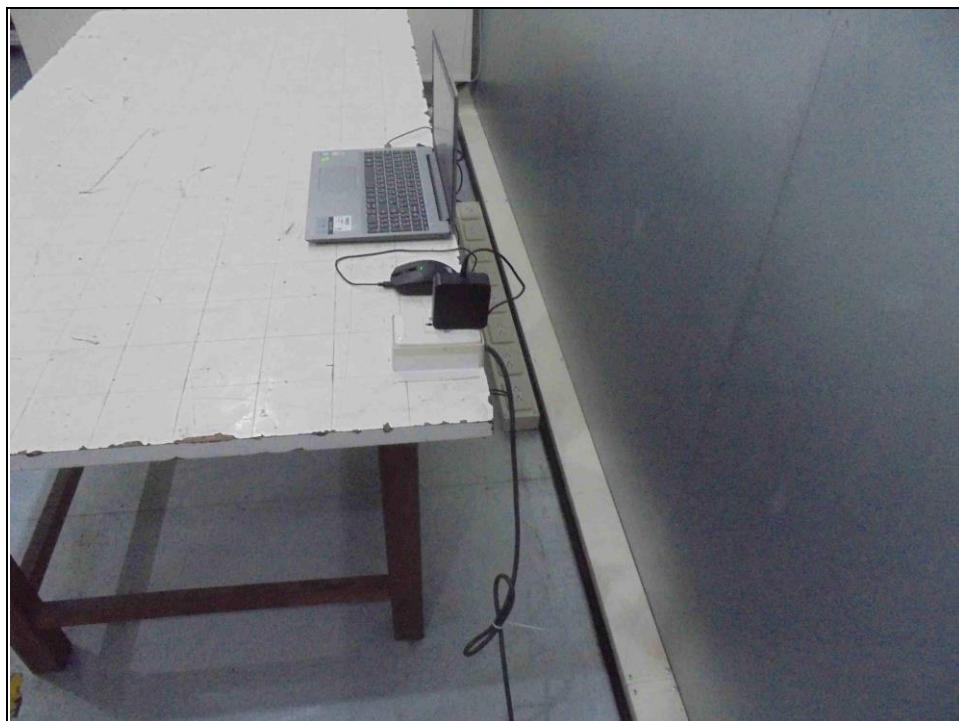
CONDUCTED EMISSION TEST (Mode C)
