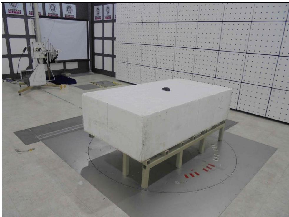
RADIATED EMISSION TEST (Mode B)
