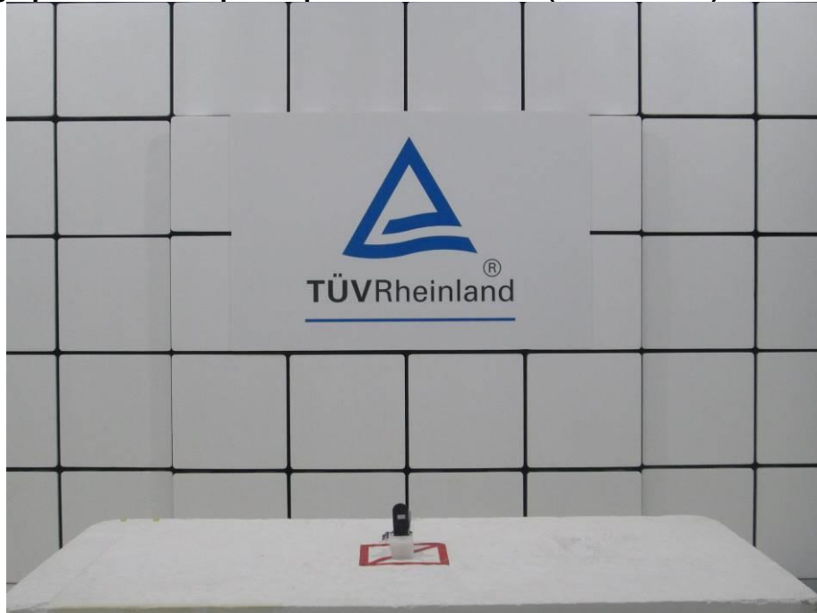
Photograph 1: Test Setup for Spurious Emissions (Front View 1)
