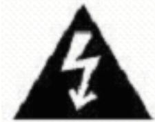
The Lightning flash with arrowhead symbol, with an equilateral triangle is intended to alert the user of the presence of uninsulated dangerous voltage within the product's enclosure that may be of sufficient magnitude to constitute a risk of electric shock to persons.
