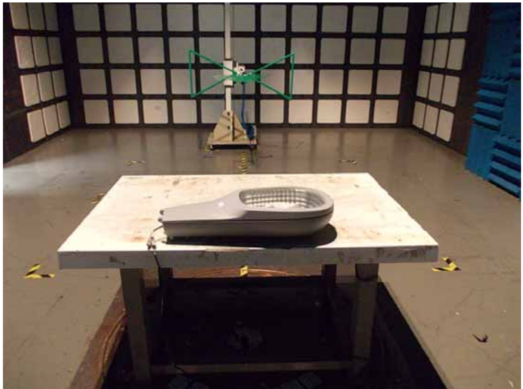
BACK VIEW OF RADIATED EMISSION TEST
