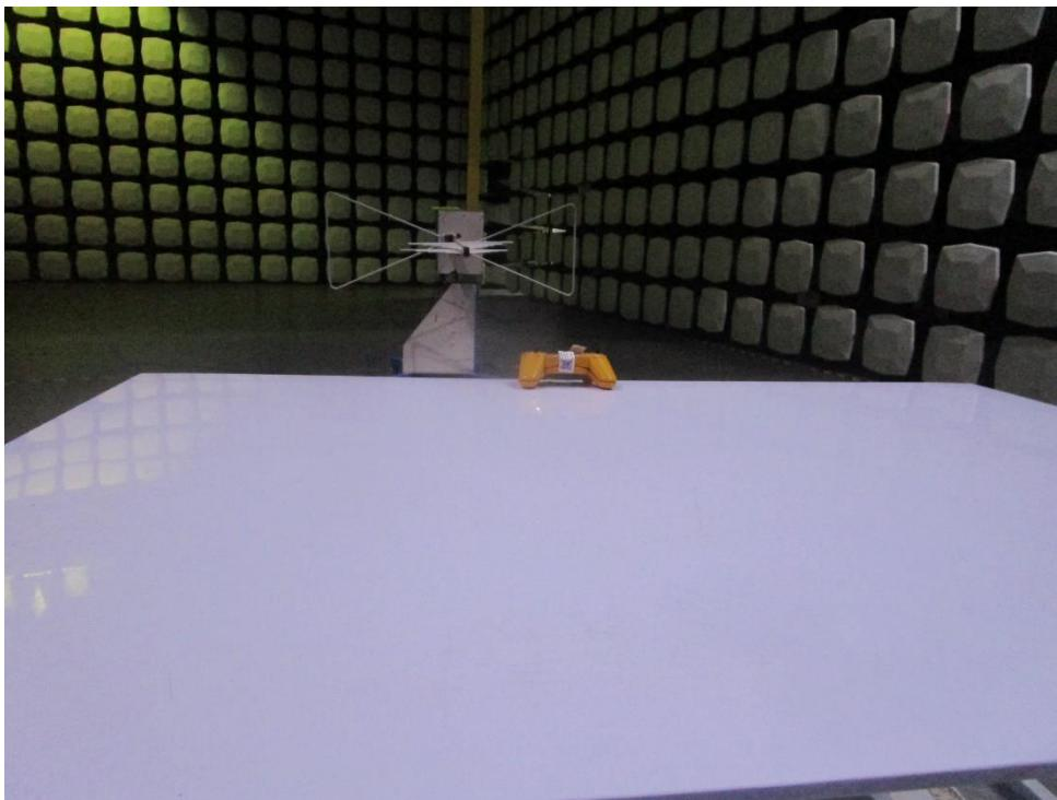
**Radiated Emissions (above 1GHz)**
