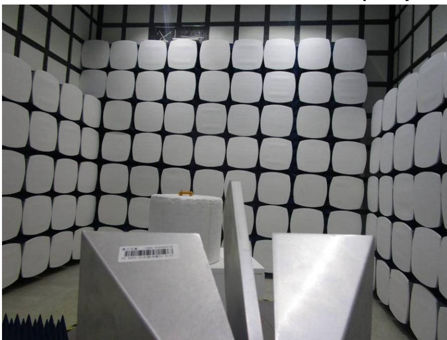
**8.3 Radiated Emissions Test Setup (30MHz~1GHz)**
