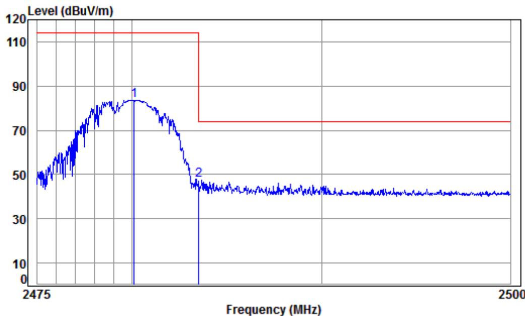
Mode:a; Polarization:Vertical; Modulation Type:GFSK; Channel:High
