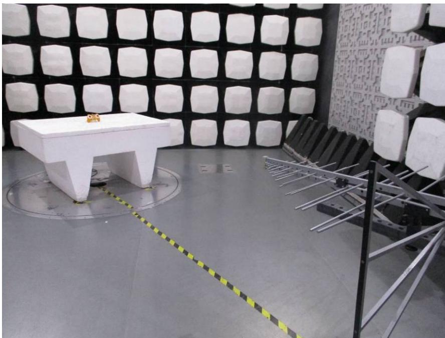
**8.4 Radiated Emissions Test Setup (Above 1GHz)**
