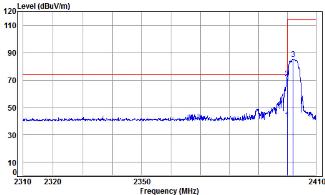
Mode:a; Polarization:Horizontal; Modulation Type:GFSK; Channel:High
