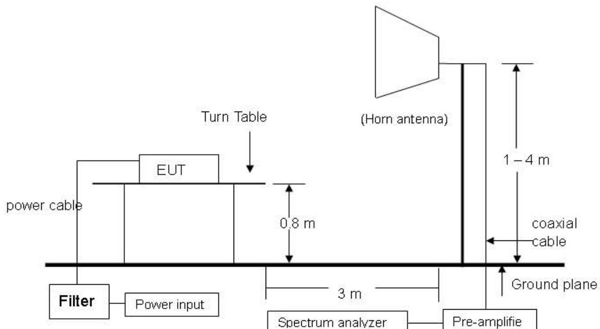
**NOTE:** The EUT system was put on a wooden table with 0.8m heights above a ground plane.
