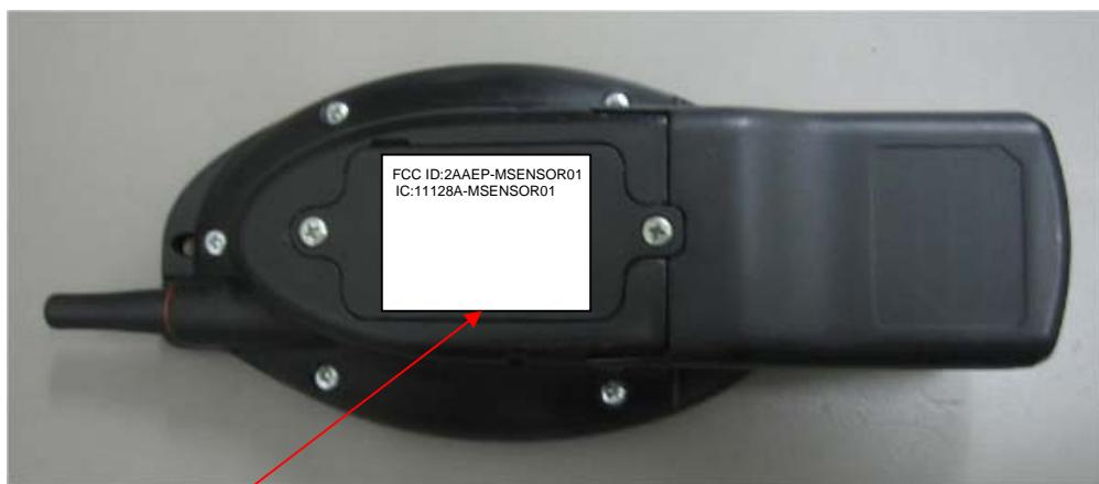
Label with **FCC ID:2AAEP-MSENSOR01** and **IC:11128A-MSENSOR01** will be located at the rear side panel. The statement according to FCC part 15 §15.19(a)(3) is placed in User Manual, page 53 (Application exhibit User\_manual\_24194).
